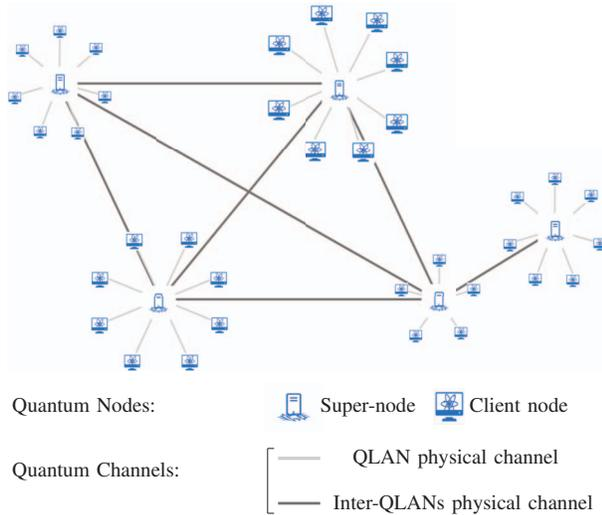
Fig. 1: Schematic representation of the considered quantum network architecture. The network comprises several Quantum Local Area Networks (QLANs). Within each QLAN, a super-node generates and distributes resources – namely, multipartite entangled states – to a set of quantum nodes – referred to as *clients* – with a star-like topology. Inter-QLAN connectivity is enabled by point-to-point quantum channels interconnecting different super-nodes.
