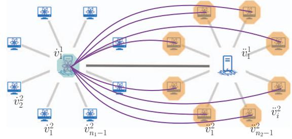
(b) Clients hand-over artificial topology discussed in Cor. 1: an artificial star topology among the same set of nodes of Fig. 4a, but centered at a super-node of a different QLAN.
