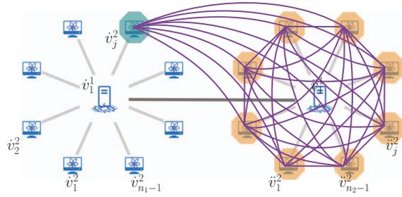
(a) *Pure peer-to-peer* artificial topology discussed in Prop 3: an artificial fully-connected topology among all the clients of the same QLAN and one client node of a different QLAN.
