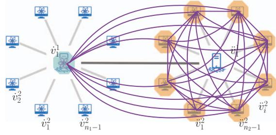
(a) Hierarchical peer-to-peer artificial topology discussed in Prop. 2: an artificial fully-connected topology among all the clients of the same QLAN and one super-node of a different QLAN.
